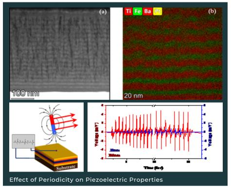
The multilayer ME composite with a periodicity between 40nm and 60nm exhibits the highest percentage of increment in d33 where there is an effective strain coupling across the interface of the two phases. The relaxation time for polarization switching of a multilayer with a periodicity of 40nm is found to be lesser compared to higher periodicities.
